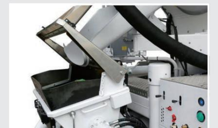
Covering for hopper in position "Own + external filling"
