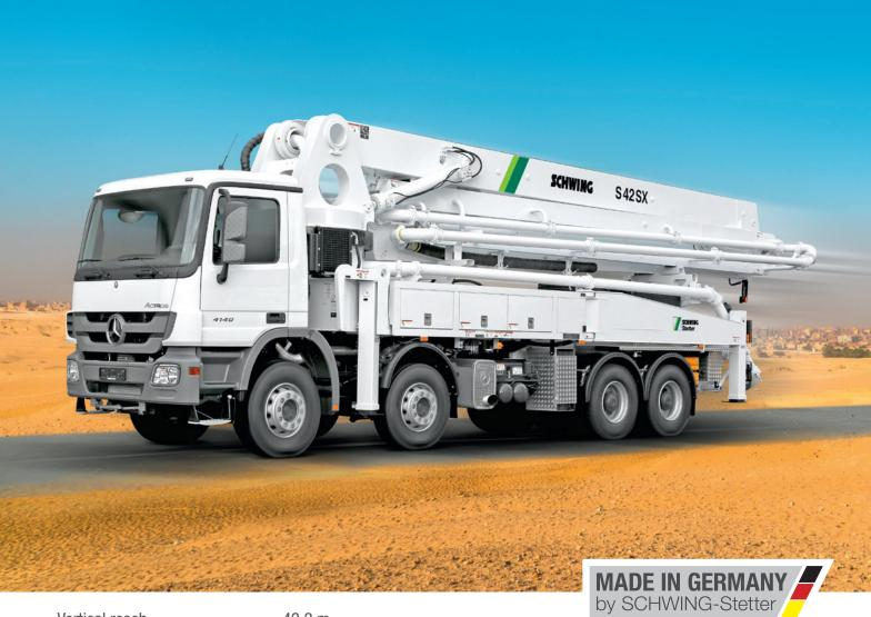
Vertical reach 42.2 m Concrete output max. 162 m³/h Pressure on concrete max. 85 bar
